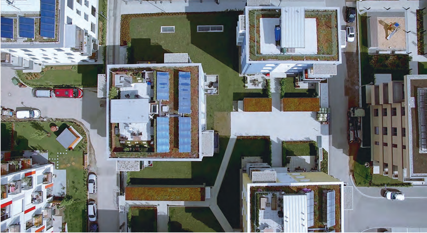
Fraunhofer ISE develops complete solutions for climate-neutral buildings, neighborhoods and municipalities. The photo shows the Gutleutmatten quarter in Freiburg, where distributed solar thermal systems were integrated into the local heating network.
