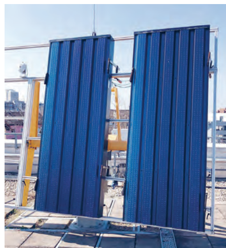
Solar collectors on the outdoor test stand.
