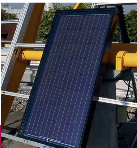
Covered PVT collector with a low-e-coated glass cover during the performance test on the outdoor test facility of TestLab Solar Thermal Systems at Fraunhofer ISE.
