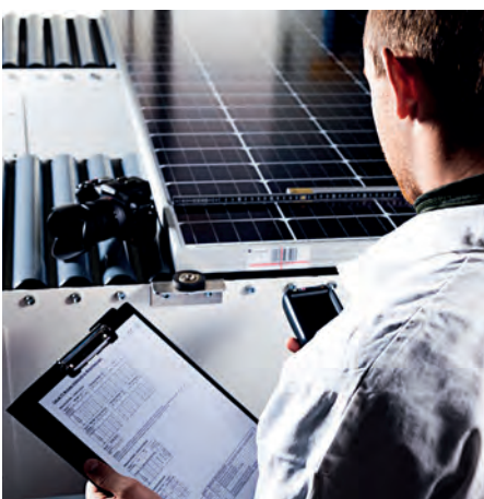
Initial inspection of a PV module.
