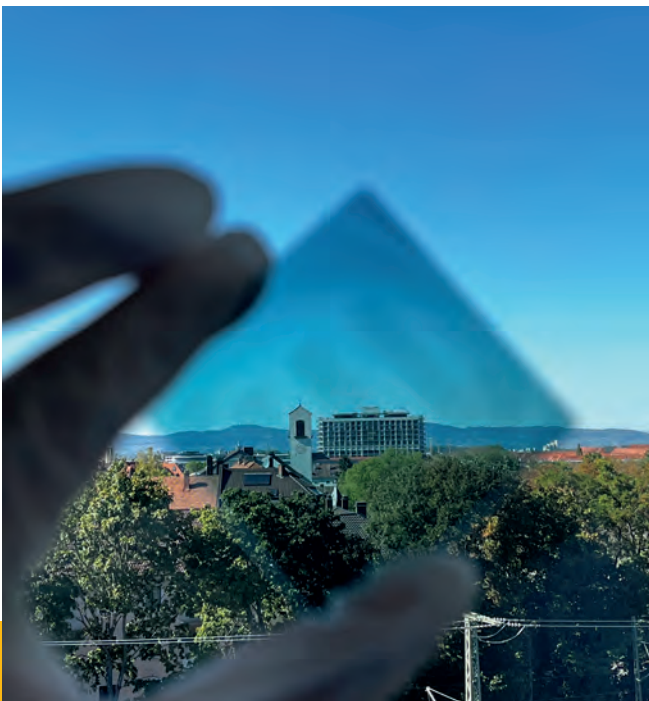
Organic solar cell with high visible transmittance.
